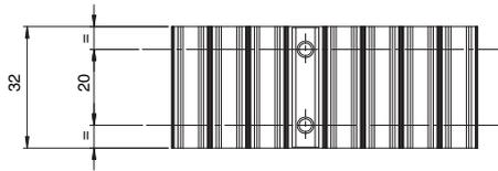
**TAS150** - suitable for AT10 profile, 50 mm wide, two pins at 25 mm centre distance
