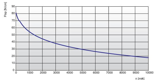
The specific load  $F_{Uspez}$  is the maximum load which one single belt tooth 1 cm wide can withstand in all operating conditions. This force is related to the drive rpm. The total load  $F_u$  transmissible by the belt in the drive is calculated by:
