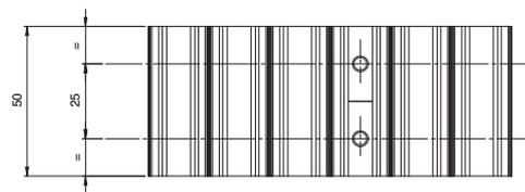
**TAS142** - suitable for AT20 and XH profile, 50 mm wide, two pins at 25 mm centre distance
