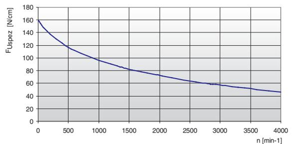
The specific load  $F_{Uspez}$  is the maximum load which one single belt tooth 1 cm wide can withstand in all operating conditions. This force is related to the drive rpm. The total load  $F_u$  transmissible by the belt in the drive is calculated by:
