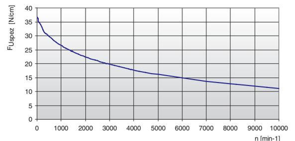
The specific load  $F_{Uspez}$  is the maximum load which one single belt tooth 1 cm wide can withstand in all operating conditions. This force is related to the drive rpm. The total load  $F_u$  transmissible by the belt in the drive is calculated by:
