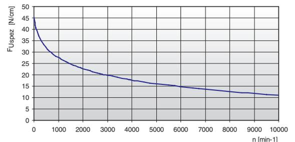
The specific load F<sub>Uspez</sub> is the maximum load which one single belt tooth 1 cm wide can withstand in all operating conditions. This force is related to the drive rpm. The total load F<sub>u</sub> transmissible by the belt in the drive is calculated by:
