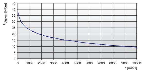
The specific load  $F_{Uspez}$  is the maximum load which one single belt tooth 1 cm wide can withstand in all operating conditions. This force is related to the drive rpm.
