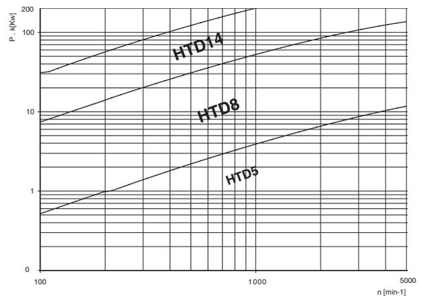
The selection graphs allows the customer to select the most suitable timing belt pitch for each belt profile and for the power to be transmitted. The rpm on the horizontal axis refers to the small pulley. The corrected power (safety factor x nominal power) is read on the vertical axis.
