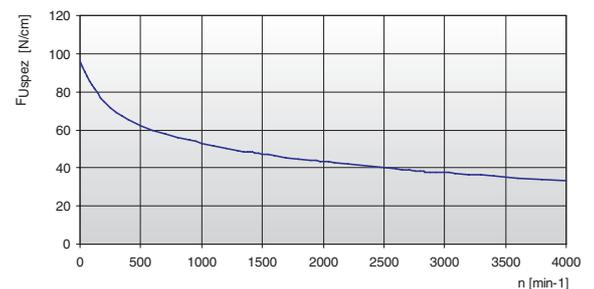
The specific load  $F_{Uspez}$  is the maximum load which one single belt tooth 1 cm wide can withstand in all operating conditions.
