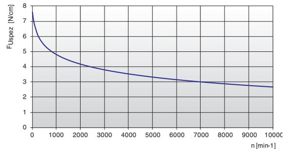
The specific load F<sub>Uspez</sub> is the maximum load which one single belt tooth 1 cm wide can withstand in all operating conditions. This force is related to the drive rpm. The total load F<sub>u</sub> transmissible by the belt in the drive is calculated by:
