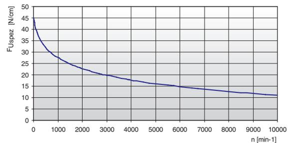
The specific load F<sub>Uspez</sub> is the maximum load which one single belt tooth 1 cm wide can withstand in all operating conditions. This force is related to the drive rpm. The total load F<sub>u</sub> transmissible by the belt in the drive is calculated by:
