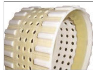
Special backings can also be machined to optimize the performance of the belts in special applications. A typical example is the hollow milling of the backing to create a “vacuum cup effect” and maximize the suction provided by water jet cut bores. In this case, perfect suction is also granted by the absence of any tension members within the vacuum areas.
