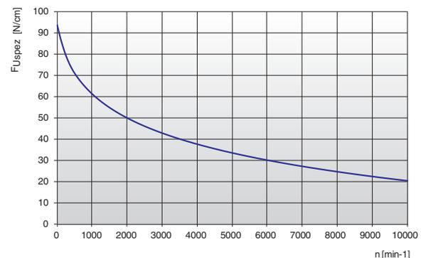
The specific load  $F_{Uspez}$  is the maximum load which one single belt tooth 1 cm wide can withstand in all operating conditions. This force is related to the drive rpm. The total load  $F_u$  transmissible by the belt in the drive is calculated by:
