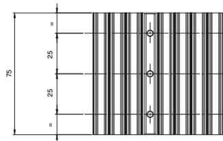
**TAS158** - suitable for AT20 and XH profile, 25-50-75-100 mm wide, number of pins multiple of 25 mm centre distance
