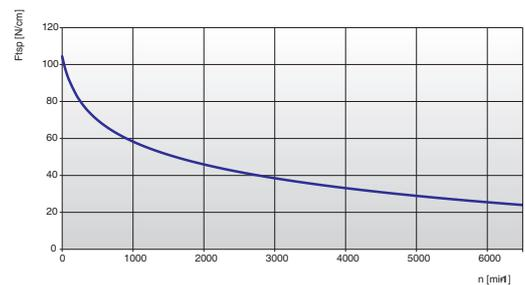
The specific load  $F_{Uspez}$  is the maximum load which one single belt tooth 1 cm wide can withstand in all operating conditions. This force is related to the drive rpm.
