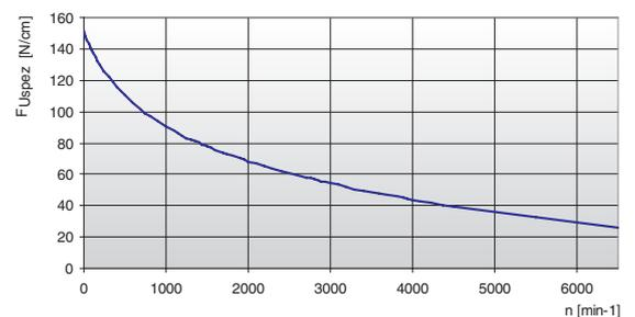
The specific load  $F_{Uspez}$  is the maximum load which one single belt tooth 1 cm wide can withstand in all operating conditions. This force is related to the drive rpm.
