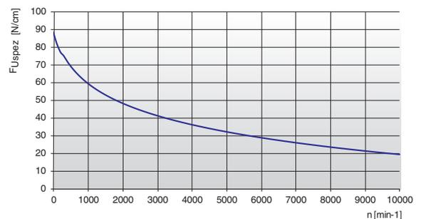
The specific load  $F_{Uspez}$  is the maximum load which one single belt tooth 1 cm wide can withstand in all operating conditions. This force is related to the drive rpm.
