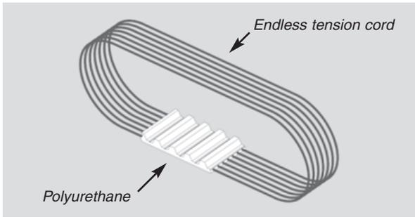
Having no splice or welding, the belts have no weak cross sections. ELA-flex SD<sup>®</sup> timing belts are therefore ideal for high speed power transmission and high load conveying applications.
